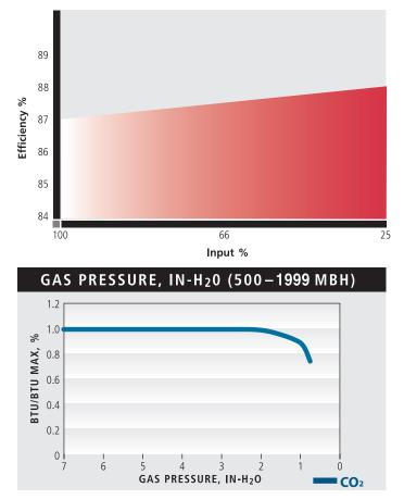
The Futera III provides high tolerance for real world conditions as it maintains 100% full input down to 2"wc.
